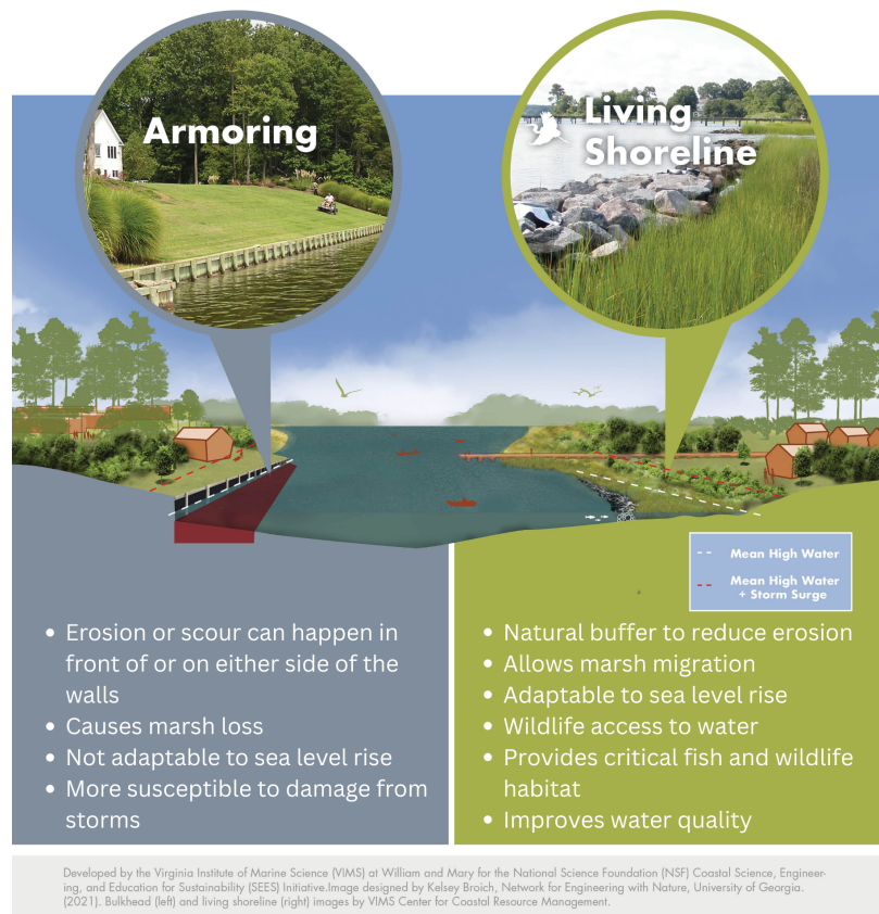
Figure 3. Living shorelines work with natural processes to attain ecosystem benefits and enhance resilience. Armoring disrupts coastal processes, reduces ecosystem benefits, and is not adaptable to changing conditions
